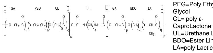
GA=poly Glycolic Acid **PEG=Poly Ethylene** UL=Urethane Linkage **BDO=Ester Linkage** LA=poly Lactic Acid
